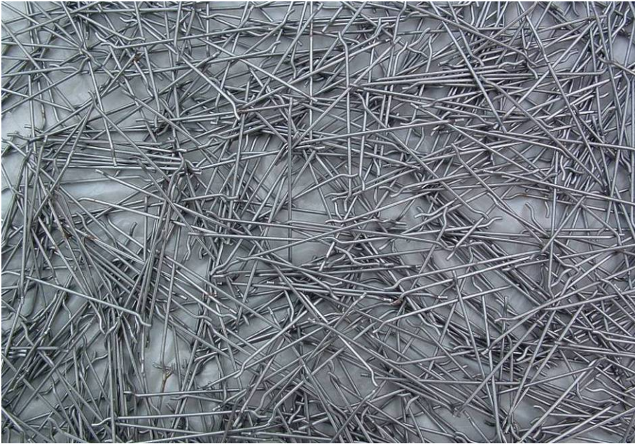
Loose hook ended fibers
